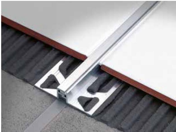
COFLEX CK technical sliding expansion joints are conceived for thin-set installations. Two metal sides interlock and slide with an internal gap of +/- 2mm, redistributing differential movement due to material compression and expansion. The profile comes assembled in a "neutral" position, held together by an elastic gasket in the lower profile section. It offers durability and high resistance to vertical loads with a modern design.
